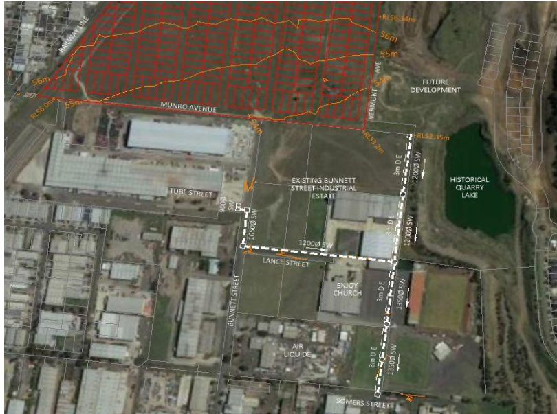
Figure 4 General Southern Catchment Stormwater Outfall Layout
